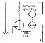
FIG. 13. Tachometer generator provides the reference signal for this speedregulation circuit.
