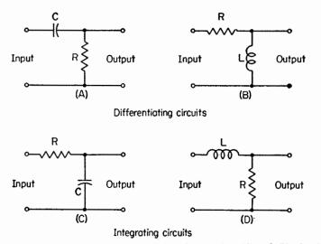
FIG. 12. Differentiating (A and B) and integrating (C and D) circuits. Integrating circuits are characterized by long time constants, while differentiating circuits have short time constants compared with the period of the applied wave.
