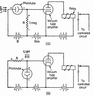
FIG. 4. Simple phototube circuits. The position of the phototube in the circuit depends on the type of operation desired. In A, the relay closes with increased illumination. In B, the relay opens with increased illumination, or it closes when illumination is decreased, depending on the initial setting.
