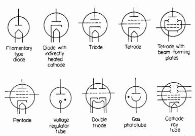
FIG. 2. Various tube symbols. Wherever a tube symbol appears in a circuit diagram, it may be considered as a signpost telling the direction of current flow, since electrons can flow only from cathode to plate in a tube.
