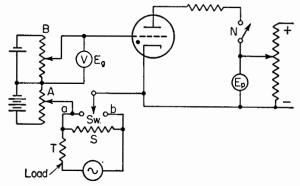
FIG. 34. Peak voltmeter using a gas triode.
