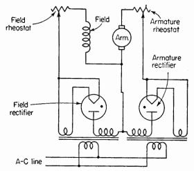
FIG. 2. Schematic for controlling the speed of a d-c motor by using gas rectifiers to convert a-c line power to direct current.
