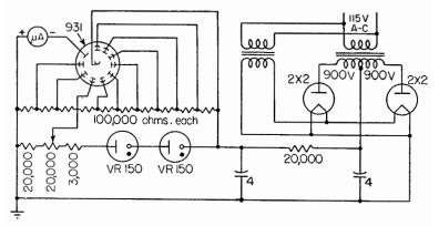
FIG. 15. Circuit for providing stable operation of a multiplier phototube by regulating part of the voltage applied to the dynodes.
