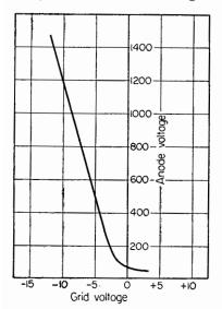
FIG. 7. Characteristics of a typical gas triode. For each value of anode voltage, there is a definite grid voltage at which the tube will "fire." If the grid is more negative than this value, no current will flow.
