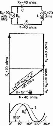
FIG. 8. In circuits containing resistance, capacitance, and inductance, the reactances counterbalance each other's effect or may cancel completely each other's effect.
