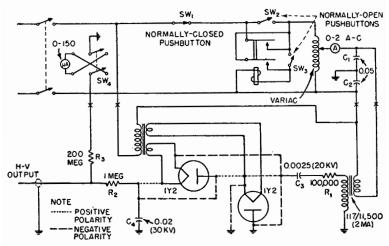
FIG. 32. Reversible 60-cycle high-voltage supply with a continuously variable output.
