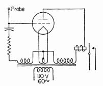
Fig. 36. Contact detector circuit. Electrons pile up on the floating grid and discharge when the probe comes in contact with a conducting object, causing the relay to operate.
