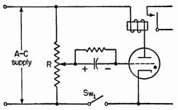
FIG. 6. Basic circuit of typical welder time-interval control.
