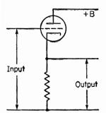
Fig. 17. Cathode-follower circuit providing very high input impedance, low output impedance, and a voltage gain less than unity.
