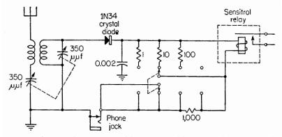
FIG. 9. Circuit using a supersensitive relay requiring no stand-by power and actuated (powered) by the energy contained in radio waves.
