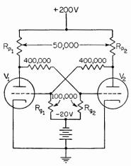
FIG. 5. Basic Eccles-Jordan pair has two completely stable sets of operating conditions.
