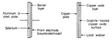
FIG. 18. Dry disk rectifiers offer numerous advantages over electron tubes in certain applications.
