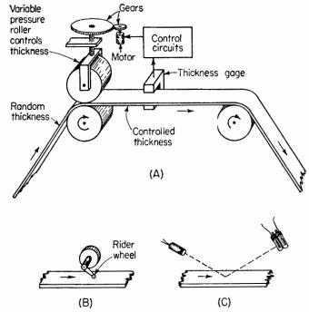
FIG. 2. Control setup for maintaining constant thickness of strip material. When the thickness gauge "tells" the control circuits that the strip is too thick, more pressure is applied to the rollers, which in turn squeeze the strip to the proper thickness.
