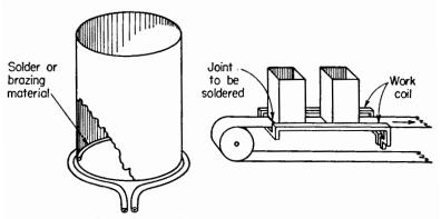
FIG. 3. When induction heating is used for soldering or brazing, the heat produced must be concentrated in a small area surrounding the proposed joint to prevent distortion of the work.
