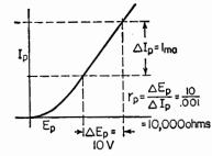
FIG. 12. The important tube parameter, transconductance or muin tual conductance, is the slope of the  $E_{\sigma}I_{p}$  line; it is the rate at which the plate current varies with the changes in grid voltage.
