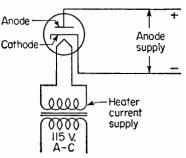
FIG. 3. Elementary diode circuit is capable of differentiating only between positive and negative voltages. Electrons will flow from the heated cathode to the plate when the plate is positive with respect to the cathode, but not when the polarity of the applied voltage is reversed.
