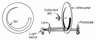
FIG. 20. Variable-slit attenuator for adjusting the illumination from a standard light source for comparison measurements.
