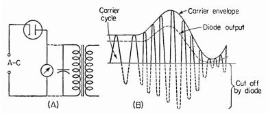
FIG. 26. Simple diode detector which cuts off one-half of the input and produces a change in the average voltage across the transformer as a function of the envelope of the modulation on the carrier.
