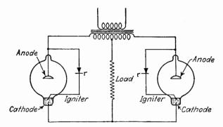
FIG. 21. Ignitron circuit especially useful in electrochemical applications.
