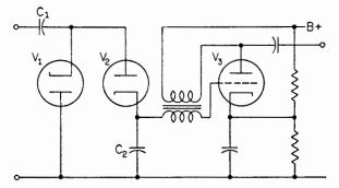
FIG. 28. Step-type counter circuit used in certain television applications.
