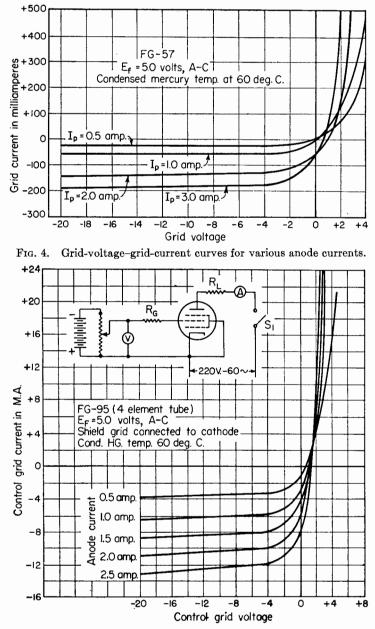
FIG. 5. Control-grid current after start of discharge in a four-element gas tube.
