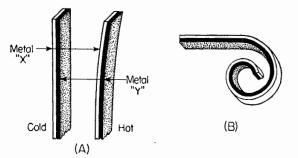
FIG. 23. Bimetallic strips transform temperature changes into mechanical changes.
