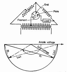
FIG. 14. Inductance and resistance phase-shift circuit.
