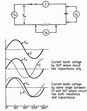
FIG. 6. In a circuit containing capacitance and resistance, voltage maximums lag current maximums by some phase angle between 0 and 90 deg.
