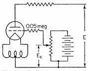
FIG. 8. Basic thyratron circuit illustrates grid control of plate current.
