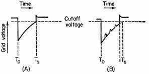
FIG. 20. Waveforms showing triggering of a free-running multivibrator.
