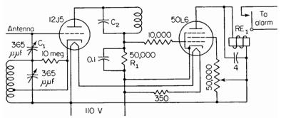
FIG. 8. Capacitance relay circuit. The relay is closed until an object approaches the antenna. This type of circuit is used widely in window displays and in burglar-alarm applications.
