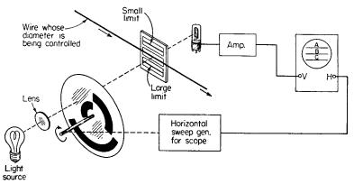
FIG. 9. Comparison system for measuring the thickness of wire continuously while the wire is traveling at high speeds. The same principle may be used to maintain constant thickness by use of proper control circuits.
