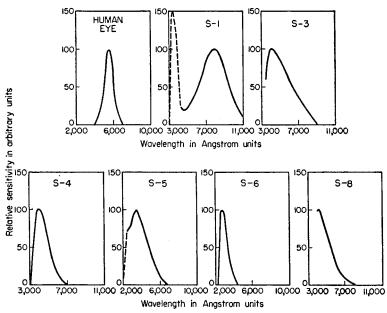
FIG. 2. Curves of the sensitivities of several phototube cathodes at different wavelengths of light.
