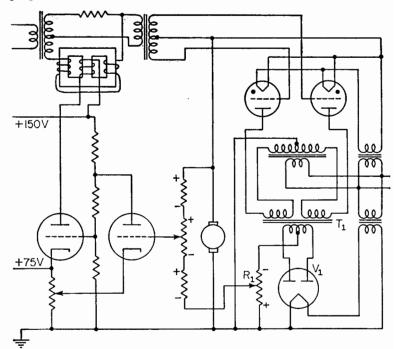
Fig. 10. Speed regulation and IR-drop compensation are provided by this circuit.
