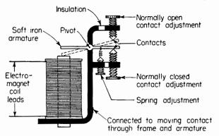
FIG. 6. Typical "telephone-type" sensitive relay construction.
