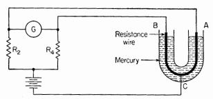
FIG. 19. The mercury shorts out sections of the resistance wire in differential fashion. Note the similarity to the circuit shown in Fig. 18.
