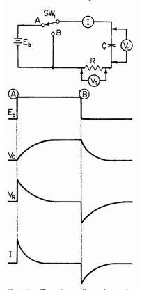
FIG. 5. Transient effects in a circuit containing resistance and capacitance. When  $SW_1$  is moved to position A, the condenser begins charging from battery. When  $SW_1$  is moved to position B, condenser begins discharging through the resistance.
