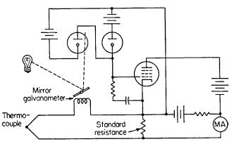
FIG. 33. Version of an automatic potentiometer system for measuring thermocouple voltages.
