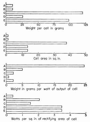
FIG. 19. Comparative data on a per-cell basis for A,  $1\frac{1}{2}$ -in. copper oxide rectifier with no coolling fins; B, same as A but with wide spacing and large cooling fins; C, copper oxide cell  $4\frac{3}{6}$  by 5 in., with oxide on both sides, assembled with normal spacing and operated with cooling fins; D, aluminumbase selenium cell with natural draft cooling; and, E, same as D except that E has an iron base instead of an aluminum base.
