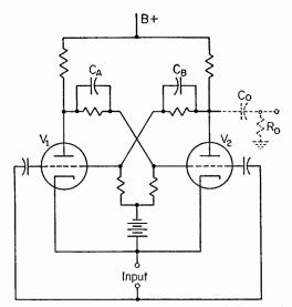
FIG. 7. Addition of commutating capacitors  $C_A$  and  $C_B$  permits the use of a single triggering input.
