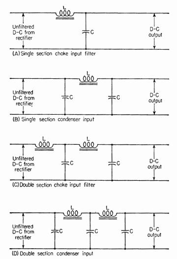
FIG. 4. Inductance-capacitance filters smooth out fluctuations in the output of rectifier circuits.
