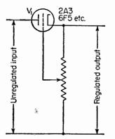
FIG. 14. Circuit of simple but effective variable-voltage regulator using standard receivingtype tubes as control elements.
