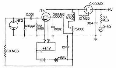
FIG. 30. Simple pulse-type high-voltage power supply for portable equipment.
