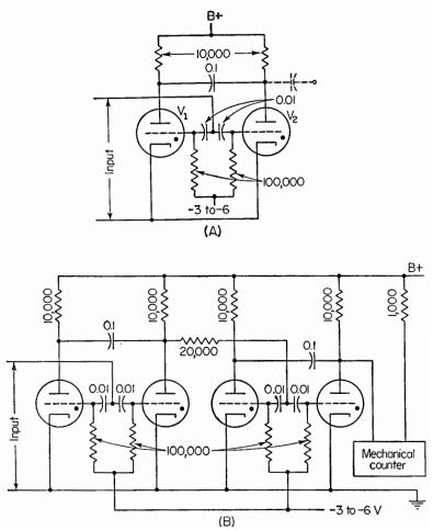
FIG. 9. Thyratron counter circuits. In B is shown how one thyratron counter circuit may be connected to a following stage.
