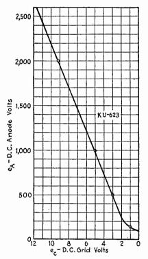
FIG. 2. Typical thyratron characteristic shows the relationship between grid and plate voltages necessary for firing.
