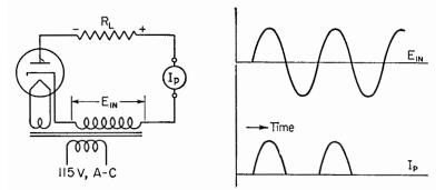
FIG. 4. Elementary rectifier circuit contains a tube, a source of a-c voltage, and a load across which a pulsating d-c voltage appears as the result of unidirectional anode current flow.
