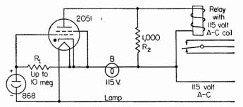
FIG. 5. Simple gas-tube relay circuit. A lamp in series with the cathode can be used as the light source for the interrupter system.
