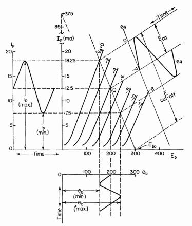
FIG. 15. Use of the load line to determine conditions in the circuit of Fig. 13.
