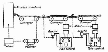
FIG. 35. System widely used for converting mechanical motion into electrical information. The slack in the web causes the core to move inside the reactor, thereby changing the reactance and speed of the conveyor motors.
