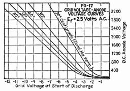
FIG. 3. Curve shows the effect of temperature on thyratron characteristics.
