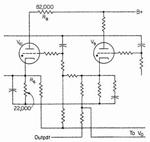
FIG. 14. Circuit showing the return of the pulse to the first stage after the count of ten.
