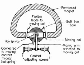
FIG. 5. A supersensitive relay is essentially a current-meter movement with contacts arranged to be opened or closed by the "needle."
