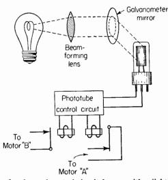
FIG. 31. Another form of control circuit for use with a light-beam galvanometer. Relays control the functions to restore balance once it is disturbed.
