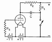
FIG. 9. Capacitor serves as a voltage-storage device in a d-c thyratron circuit.
