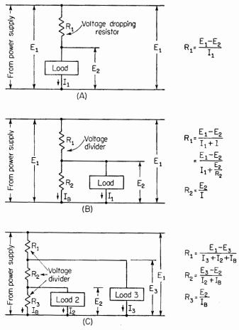
FIG. 8. When more than one voltage is to be furnished by a single d-c power supply, voltage-dropping or voltage-dividing resistors may be used.
