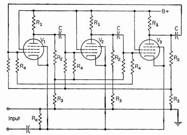
FIG. 17. Ring-of-three counter produces one output pulse for every three input pulses.
