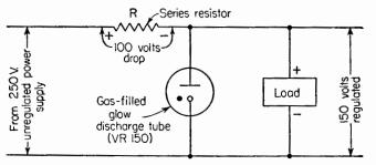
FIG. 9. Glow-discharge voltage-regulator tubes are readily available for holding constant voltages of 75, 90, 105, and 150 volts, where low current requirements exist.
