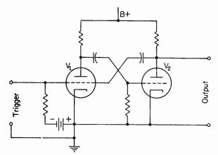
FIG. 25. Basic single-shot multivibrator undergoes one complete cycle for every pulse applied to the input.
