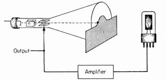
FIG. 25. A phototube and a cathode-ray tube provide a wide variety of available waveforms. The spot on the tube screen follows the contour of the opaque mask.
