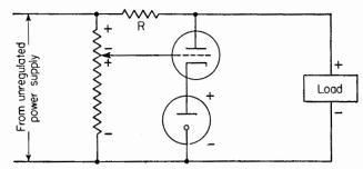
FIG. 11. Glow-discharge regulator provides fixed reference-voltage bias for the variable-voltage regulator, thus eliminating the bias battery shown in Fig. 10.
