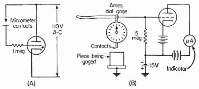
FIG. 7. Use of an electron tube for detecting mechanical contact between two metallic parts. The flow of current through the contact points is negligible when a vacuum-tube amplifier is used between the contacts and the indicating instrument.
