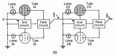
FIG. 4. Basic flip-flop circuits show counter-indication method and cascading of basic circuits for counting higher than the basic 2.
