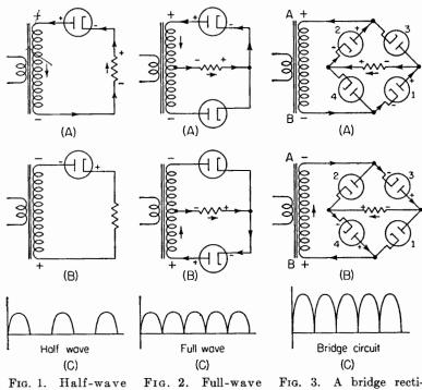
FIG. 1. Hall-wave rectifier circuit. The arrows indicate the direction of current flow. The tube conducts current when, and only when, its plate is positive with respect to its cathode.
