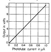
Fig. 12. Curve showing linearity of output obtained from the cathode-follower circuit of Fig. 11.
