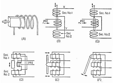
FIG. 13. Differential transformers provide a good link between mechanical and electrical phenomena.
