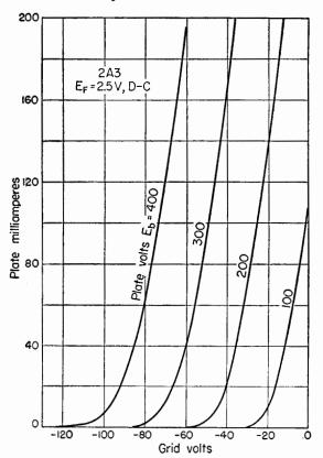
FIG. 3. Curves relating the grid voltage and plate current  $(E_g-I_p)$  of a typical triode, the 2A3.
