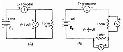
FIG. 1. Basic circuits containing series resistance and a d-c voltage source illustrate the application of Ohm's law.
