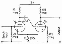
FIG. 24. Cathode-coupled multivibrator circuit.
