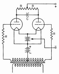
FIG. 10. Circuit showing the use of a second thyratron instead of the switch in Fig. 9 to force anode negative.
