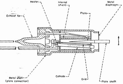
FIG. 21. Sketch of RCA 5734 triode transducer tube.
