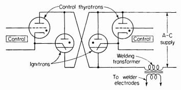
FIG. 7. Enormous values of welding current can be controlled by this circuit. Actual control is applied to the primary of the welding transformer by a combination of thyratron firing tubes and ignitrons.
