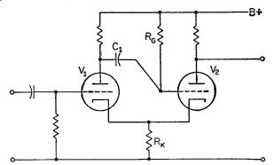
FIG. 26. Cathode-coupled single-shot multivibrator circuit.
