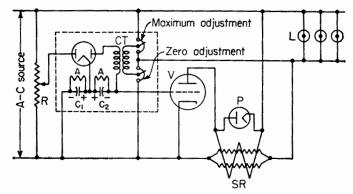
FIG. 37. Illumination-control circuit using tubes.
