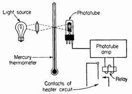
FIG. 26. Simple method for maintaining a fixed temperature. When the mercury rises in the tube, it cuts off the light to the phototube. The photo-tube circuit releases the relay and turns off the heater.
