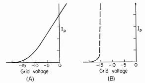
FIG. 1. Typical characteristics of vacuum tubes (A) and gas tubes (B).
