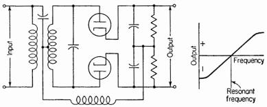
FIG. 24. Discriminator circuit. The output is a function of the variation in frequency of the applied input.
