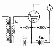
FIG. 5. Triode with a source of alternating voltage in series with steady grid bias. Alternating currents produced in the anode circuit correspond to the alternating grid voltage.
