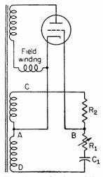
FIG. 7. Basic phase-shift circuit shows a bridge configuration.
