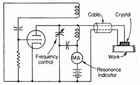
FIG. 5. Basic circuit of an ultrasonic thickness gauge.
