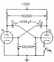
FIG. 19. Symmetrical multivibrator circuit. This circuit has two unstable sets of operating conditions, and it automatically flips back and forth between them.
