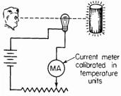
FIG. 25. Basic optical pyrometry arrangement.
