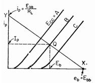
FIG. 11. Construction of the load line by which all the voltages and currents in **a** triode amplifier circuit may be obtained.  $E_{cc}$  is the fixed grid bias;  $E_{bb}$  the fixed plate voltage.
