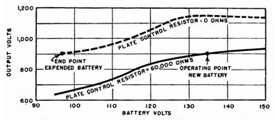
FIG. 31. Output curves for the supply shown in Fig. 30 show the effects of an aging battery.
