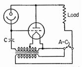
FIG. 15. Plate current is varied by changing phototube current.
