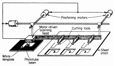
FIG. 12. Photoelectric contour follower. Cutting tools automatically trace out the contour represented by the paper pattern on the table.
