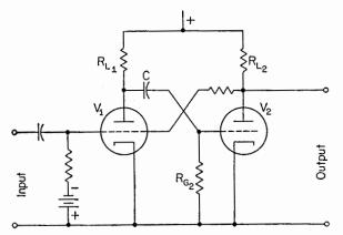
FIG. 27. Alternate single-shot multivibrator circuit capable of square-wave output.
