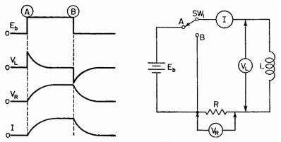
FIG. 2. Transient effects in a circuit containing resistance and inductance. When  $SW_1$  is moved to position A, the battery voltage is impressed across the coil and its resistance. When  $SW_1$  is moved to position B, the battery is disconnected and the inductance is shorted.
