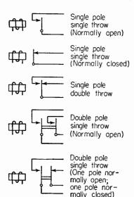
FIG. 2. A wide variety of contact arrangements is possible. Several typical combinations are illustrated here. of this device, which merely consists of an extra pair of contacts that are closed when the relay is energized, the relay may be energized by a momentary switch and held in its energized position until the coil circuit is interrupted by an auxiliary switch (reset) that is normally closed.
