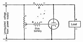
FIG. 10. Simple variable regulator tube maintains constant load voltage by varying the current through the series resistor R.
