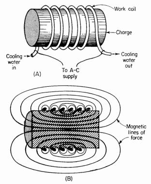
FIG. 1. Basic induction heating setup. High-frequency alternating current passed through the coil heats the metallic charge. The depth of heating depends on the frequency of the heater current.
