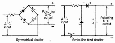
FIG. 25. Selenium rectifiers may be used in the voltage-doubler circuits shown to produce approximately twice the voltage of the line.
