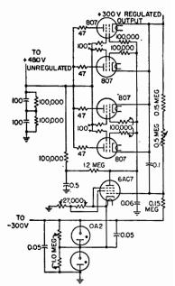
Wide-range voltage regu-FIG. 16. lator provides constant voltages from a few volts to several hundred volts.
