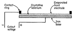
FIG. 14. Cross section of a Weston Photronic cell.
