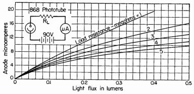
FIG. 12. Typical phototube characteristics.
