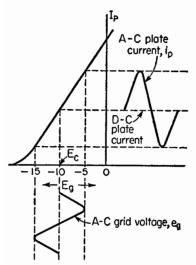
FIG. 6. With each variation in grid voltage there is a variation in plate current. Here, capital letters indicate steady or d-c values; small letters are the a-c components.
