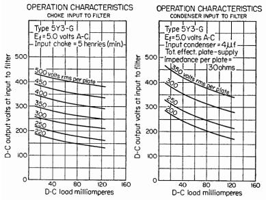
FIG. 6. Typical curves provide all essential information for figuring the performance or rectifier tubes. This example (from the "RCA Receiving Tube Handbook") shows characteristics for the 5Y3G high-vacuum dual-diode rectifier tube.
