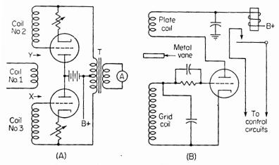
FIG. 10. Reluctance thickness gauges. The coupling between coils is varied by the presence of metal.
