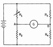
FIG. 18. Bridge circuit for measuring unknown resistance values.
