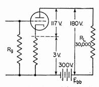
FIG. 7. Complete triode circuit with voltage division between the tube and load for a steady plate current of 6 ma. Here the plate current flowing through a 500-ohm cathode resistor,  $R_{k}$ , produces a 3-volt drop which may be used as grid bias. Of the 300 volts from the plate battery, 180 appears across the load, 117 between the plate and cathode, and 3 volts between the cathode and ground. No current flows through  $R_{g}$ , and there is no voltage drop across it.
