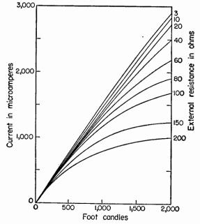
FIG. 15. Characteristics of a Weston Photronic cell with various values of external resistance.
