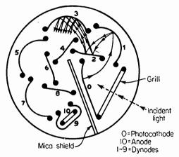
FIG. 13. Schematic of the multiplier phototube with its cathode, nine dynodes, and final anode or collector.
