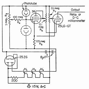
FIG. 10. Simple phototube circuit using conventional receiving-type tubes to obtain good sensitivity and stability.
