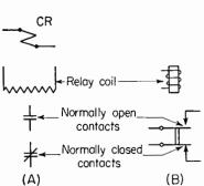
FIG. 1. The symbols for relays shown in A are used extensively in industrial power circuits; those in B, in periodicals dealing in general electronic circuits.
