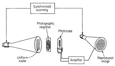
FIG. 23. This simplified television system uses a phototube to pick up variations in light from a cathode-ray-tube flying-spot scanner.
