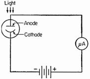
FIG. 3. Basic phototube circuit. The battery provides current, and the microammeter measures changes brought about by different light intensities on the phototube cathode.
