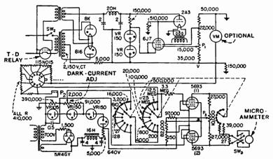
FIG. 16. Complete circuit of a multiplier-phototube unit with attenuators and a stable amplifier.
