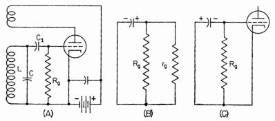
FIG. 25. Simple feedback oscillator in which a voltage is returned to the input from the output by means of a plate coil coupled to the grid inductance. In B and C are the effective input circuits for determining grid bias by means of grid current.
