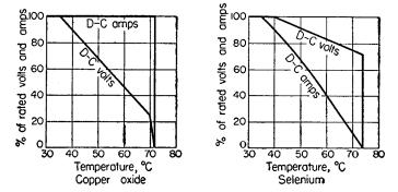
FIG. 23. Reduced rating curves for unusual temperature conditions.
