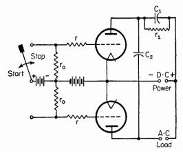
FIG. 18. Industrial circuit using two thyratrons.
