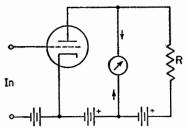
FIG. 28. Simple triode vacuumtube voltmeter in which any change in the grid voltage produces a change in the plate current. The additional battery and resistor are adjusted so that zero current flows through the meter when no grid signal is applied.
