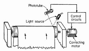
FIG. 11. Phototube setup for maintaining the correct position of a strip on a roller.
