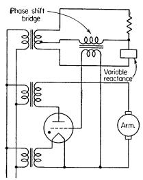
FIG. 4. Diagram of means for retarding the phase of thyratron grid voltage for varying the current supplied to the motor armature.
