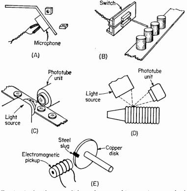
FIG. 1. A microphone or switch may be arranged to convert some mechanical phenomenon into an electrical signal for counting purposes, as shown in A and B. In C and D a phototube circuit detects movement and creates the counting signal. A means for obtaining electrical signals for counting revolutions of rotating machinery is shown at E.
