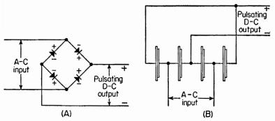
FIG. 26. Bridge circuits are frequently used in conjunction with dry disk rectifiers.
