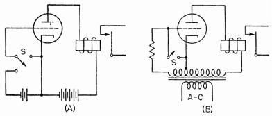
FIG. 7. Use of electron tubes permits control of fairly rugged relays by extremely low power switches.
