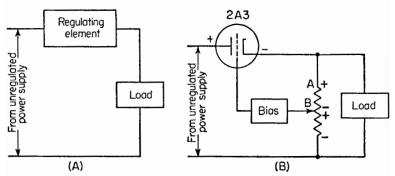
FIG. 12. Voltage-regulator circuit maintains constant load voltage by varying the resistance of the control tube in series with an unregulated source.
