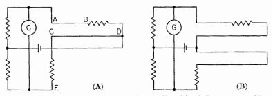
FIG. 20. Two schemes for compensating for disturbing influences caused by variations in conditions between an unknown resistance element and the measuring equipment.
