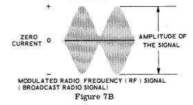
the form of swells of energy. The audio information is contained in these swells of RF signal; first there is very little energy, and then there is a lot of energy. To put it another way, the audio information exists in the way the RF signal changes in amplitude.
