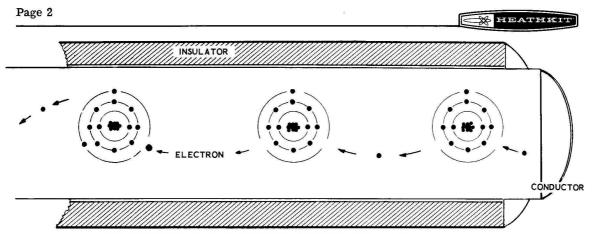
A GREATLY ENLARGED VIEW OF THE ELECTRONS FLOWING FROM ATOM TO ATOM IN A LENGTH OF WIRE  $Figure \ 1B$
