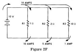
If the total or overall resistance for the parallel circuit were calculated it would be equal to a single resistor that would allow the same total amount of current to flow through it alone as now flows from the battery through all three current paths. This total resistance for a parallel circuit can be calculated using the formula  $\frac{1}{R}$  TOTAL =  $\frac{1}{R_1} + \frac{1}{R_2} + \frac{1}{R_3}$ See the example shown in Figure 2G.
