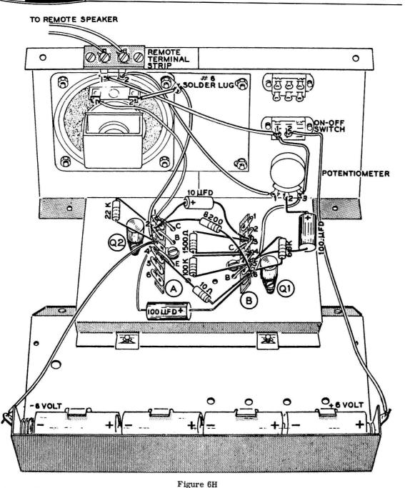
( ) Turn the ON-OFF switch ON and notice the sound has once again become drastically changed (usually the sound will be com-pletely cut off in this case).
