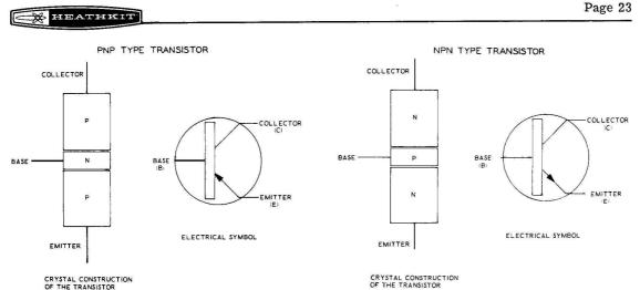
CRYSTAL CONSTRUCTION OF THE TRANSISTOR
