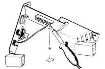
PROP THE CHASSIS UP SO THAT SOLDER WILL FLOW FREELY FROM THE LUG
