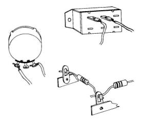
wet the wire is sufficient. Apply a small amount of solder to the place where the wire is to be connected (sometimes, solder from a previous connection will work here). Now hold the wire and the tip of the soldering iron against the terminal until solder flows between the two. Hold the wire so that it does not move until the joint cools, and the connection is complete.
