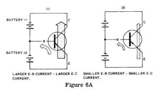
Since the large Collector currents are often 100 times as large as the smaller Base currents it is almost as if the small Base current were opening and closing a valve between the Emitter and Collector. A larger Base current would compare to opening the valve wider, and letting a <u>larger</u> Collector current flow through the transistor. A smaller Base current would compare to closing the valve, causing a smaller amount of Collector current to flow through the transistor.
