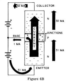
To make the transistor operate properly, the batteries are connected so that the Emitterto-Base junction has <u>forward bias</u> applied to it, and the Base-to-Collector junction has <u>reverse bias</u> applied to it. Because the Base crystal is actually constructed so that it is very
