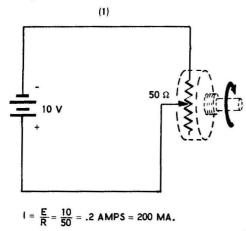
When the shaft is turned, the resistance between the center lug and both outside lugs changes. For this lesson, only two of the variable resistor terminals will be used, the center terminal, and either one of the other terminals.
