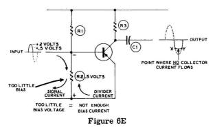
Figure 6E shows the circuit condition where the bias voltage across resistor R2 is cancelled out. The bias current flows up through resistor R2 as it did before. During the positive half-cycle of the input waveform, the signal current attempts to flow down through resistor R2 with the result that it bucks up against the bias current and cancels some of it.
