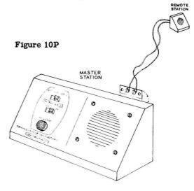
As described in Lesson VIII, some of the output of the (intercom) amplifier was connected from the output speaker back to the input (microphone) speaker - resulting in the oscillation. Note that this oscillation continues in both positions of the LISTEN-TALK switch.
