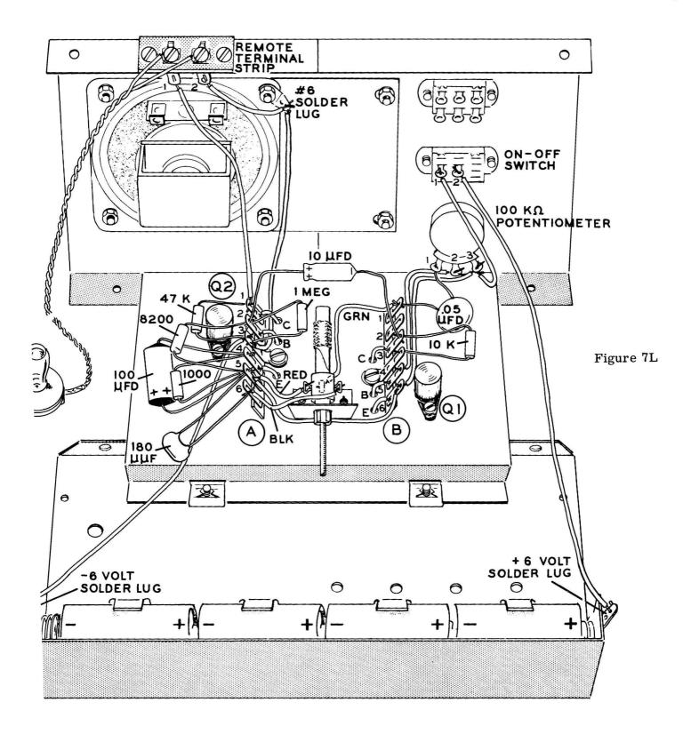
REMOTE TERMINAL STRIP  $\emptyset$ 0 Ø 0 A 6 Ø#6 SOLDER 3 5 8  ${\bf \Box}$ LUG ON OFF SWITCH 8 8 吸图 2 6 3 100K .01 µFD POTENTIOMETER IOK .005 .005 0 0 С 1004 Q B 8200 C E TO EARPHONE B 0 0 202 J. Θ 0 \_)| .01 µfd EARPHONE -6 VOLTS II MEG 3 100 K 8200 +6 VOLTS 0 ●)| .005 µfd QI Q2 22 K ł ł \$100 к ∳ ON-OFF SWITCH S 10 K
